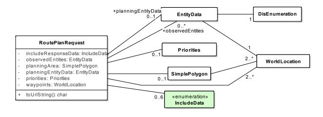
**Figure 9:** Description of the request to the route planning service. A request includes way points, data for the planning entity, and a bounding area for path planning. It also includes data for other relevant entities such enemies within the planning area. IncludeData is an enumeration for what kind of additional data to include in the response, for example speed along the route.
