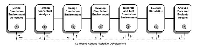
Figure 4: Distributed Simulation Engineering and Execution Process (DSEEP), main steps [14].
