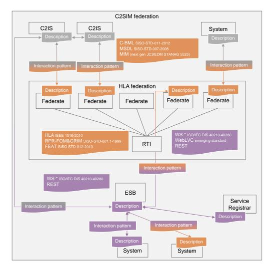
Figure 7: Reference Hybrid Architecture for C2SIM federation
